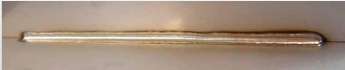
TIG DC continuous fillet weld without additional material by
